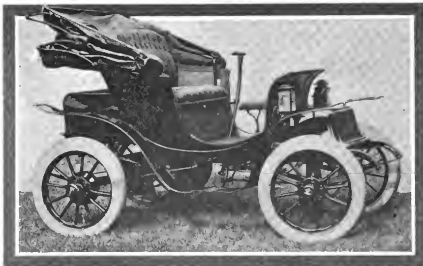
Fig. 2—Model 17-D Victoria-Phaeton with extra seat, divided battery of the Exide type, interlocking control and standard finish
